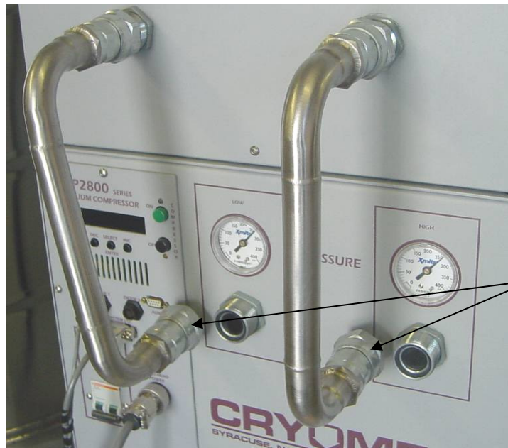
Figure 8-2: Aeroquip® couplings disconnected from the compressor
